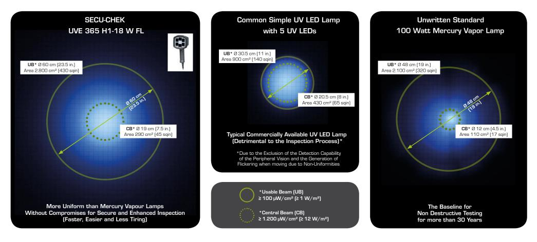
SECU-CHEK UV LED Lamps are Especially Designed for NDT and Offer TOTAL UNIFORMITY of the Beam with Soft Drop-Off at the Edges as Required for Fluorescent Magnetic Particle Testing (MPI) and Fluorescent Penetrant Testing (FPI) by Leading Aerospace Standards like Airbus AITM 6-1001, ISSUE 11 and Rolls Royce RRES 90061.
